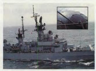
Starboard side of *USS Worden* after she absorbed two Shrike anti-radar missiles fired by a "friendly" jinked-out jet jockey returning from a mission over Halphong. *Inset: Worden*'s fire control radars took hundreds of shrapnel hits — protecting all but one of the 50 men in CIC during the errant attack.
